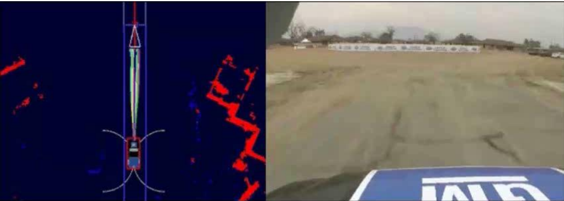
planning on 4D ( \langle x,y,orientation,velocity \rangle ) multi-resolution lattice using Anytime D* [Likhachev & Ferguson, '09]
