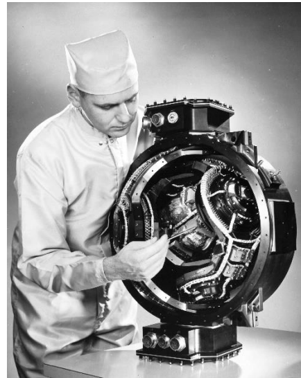
ST-124 Inertial Guidance Platform used in the Saturn V, 1960s
